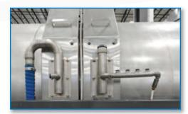
Water and chemistry are injected at this location with the chemistry added above the water level for proper and thorough mixing.
