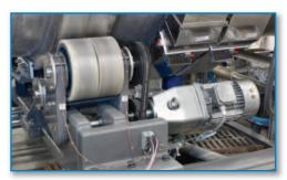
The drive system of the Braun Tunnel Washer is simple, rugged and reliable. There are no chains that may wear or break. The four drive motors are readily accessible and provide an error-free friction drive system.
