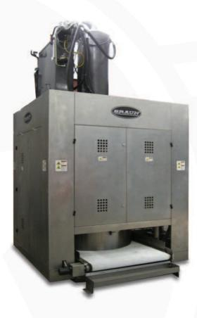
Features a quick cycle time with adjustable pressure ramp rates to obtain maximum pressure in a short time if desired. Braun SmoothFlow Single-stage Batch Extraction Presses are manufactured for 100% cotton, polyester/cotton-blended fabrics, 100% synthetics, and special textile items such as incontinence pads.
