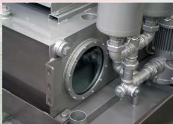
Sight glass on backside of tank
